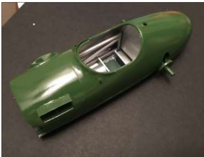
Here it is in place after paint. I also lined the cockpit with the inside of a Coke can to replicate the aluminum finish of the interior.
