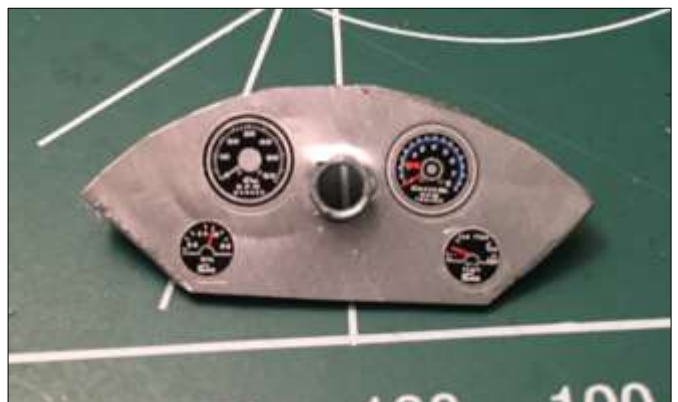
I made a new instrument panel with the aluminum from the can and fitted some spare decals.
