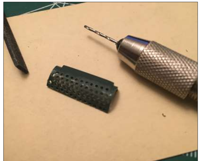
Drilling out the exhaust shroud
